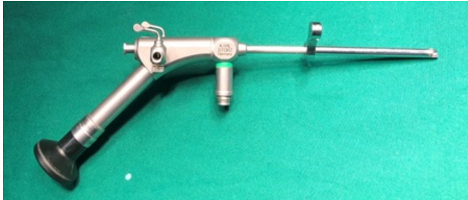
Fig. (3). Photo of a 4-mm Storz cervical endoscope with an inner central working channel measuring 2.7 mm accommodating 2.5 mm instruments. The endoscope has an ocular attachment for commonly available CCD video cameras. The light is attached to the bottom quick connect. The endoscope has two stop-cocks for irrigation fluid and suction channel attachments. The working sleeve has a beveled tip and a vane to help manipulate the working cannular during surgery.
