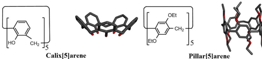
Fig. (1). Comparison of chemical structures of pillar [5]arene [P5A] and calix [5]arene. (Adopted with permission from ref. 8).
