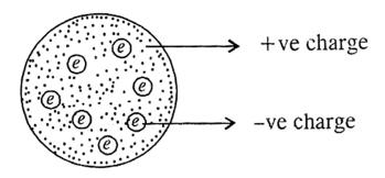
Fig. (3.1). Schematics of an atom as the smallest unit of matter.
