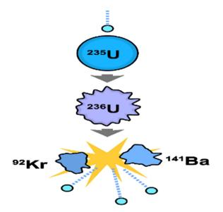
**Fig. (6.1).** An illustration of an induced nuclear fission event. Courtesy: "Wikimedia Commons." Originally created by Fast fission in Illustrator. Source: https://commons.wikimedia.org/w/index.php?curid=486924.
