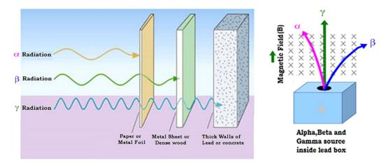
Fig. (7.1). Schematics of Alpha, Beta and Gamma rays.
