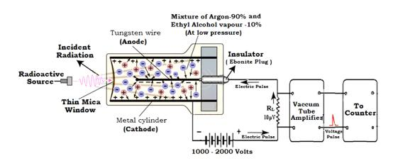
Fig. (4.1). Schematics of G. M. Counter.
