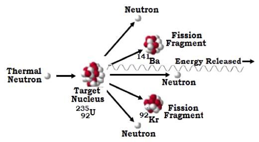
Fig. (2.1). Nuclear Fission Mechanism.
