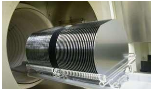
Fig. (3). Insertion of pure silicon wafers into a thermal oxidation chamber stacked in a slotted quartz wafer holder
